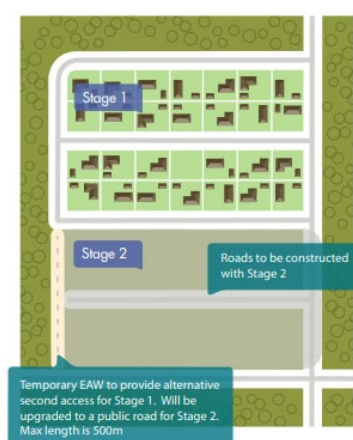
Figure 22: Example of an emergency access way
