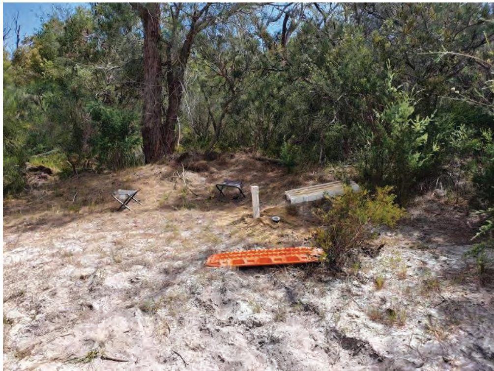
Photograph 7: Standpipe within IT09 to carry out infiltration test
