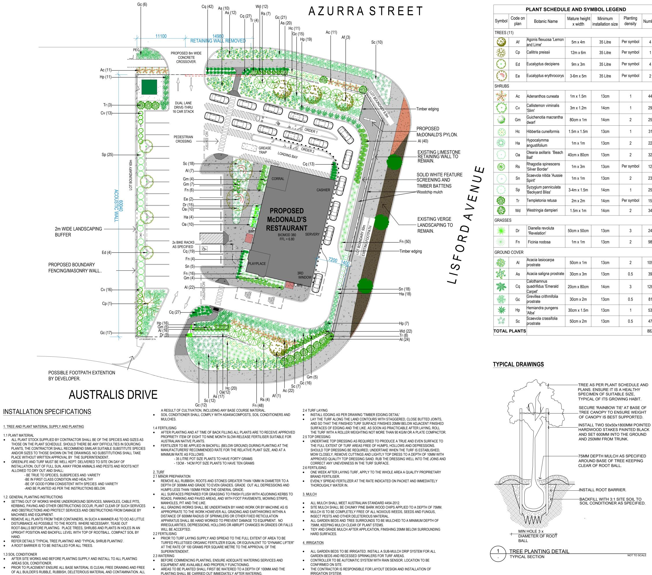
OF ALL BUILDER'S RUBBLE, RUBBISH, DELETERIOUS MATERIAL AND CONTAMINATION. ALL AREAS CONTAMINATED BY THE BUILDER OR OTHERS SHALL BE REMOVED AND REPLACE WITH CLEAN FILL SAND TO THE APPROVAL OF THE SUPERINTENDENT. PLACE SOIL CONDITIONER TO A DEPTH OF 15MM OVER THE FULL EXTENT OF AREAS TO BE
