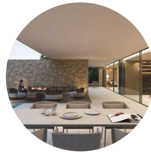
④ Deep Overhang for solar control
