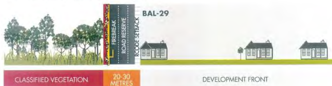
Figure 16: A reduced separation distance may necessitate increased construction standards It may be possible to reduce the minimum distances, for example by increasing the construction standard of the building – in this example the building would need to be constructed to BAL-29
