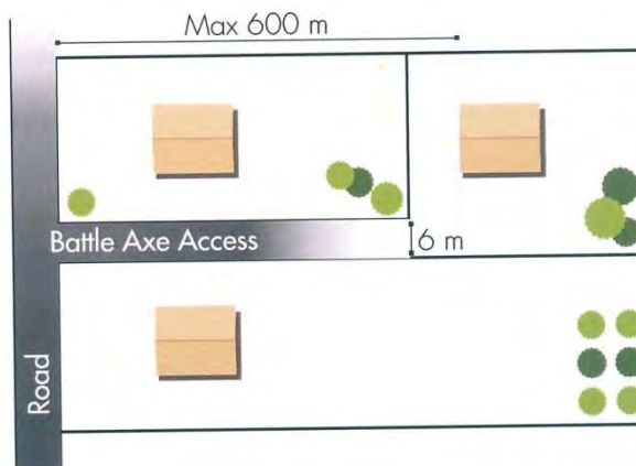
Figure 19: Minimum design requirements for a battle-axe
