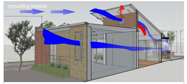
Maximising the flow of cooling breezes through a home is an essential component of passive design. Cooling breezes help to flush excess internal summer heat build up, providing effective cooling in most climate types. In addition to the cooling benefits, adequate ventilation is important for maintaining indoor air quality. By effectively using a number of 'passive cooling' techniques it is possible to design a home to be comfortable in summer without air conditioning.
