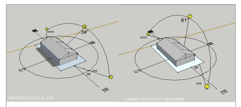
The direction your home faces is the starting point of solar passive design. Solar orientation involves placing a home on the site in such a way that the home takes full advantage of the sun's natural heat and/or cooling breezes.
