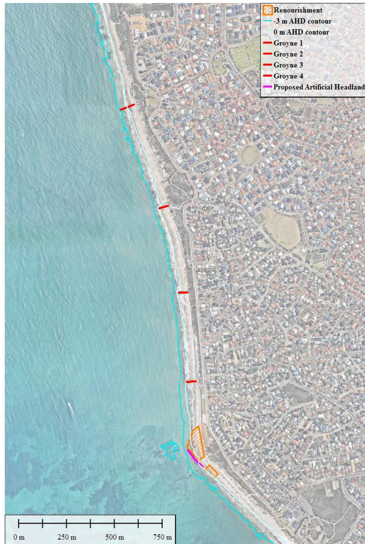
Figure 2-1 Conceptual Layouts for (a) Option 9. Groynes 1 to 3 are unchanged in length; extended artificial headland extended shown by the purple line; Groyne 4 new structure. (b) Option 10. Red lines indicate modelled structures
