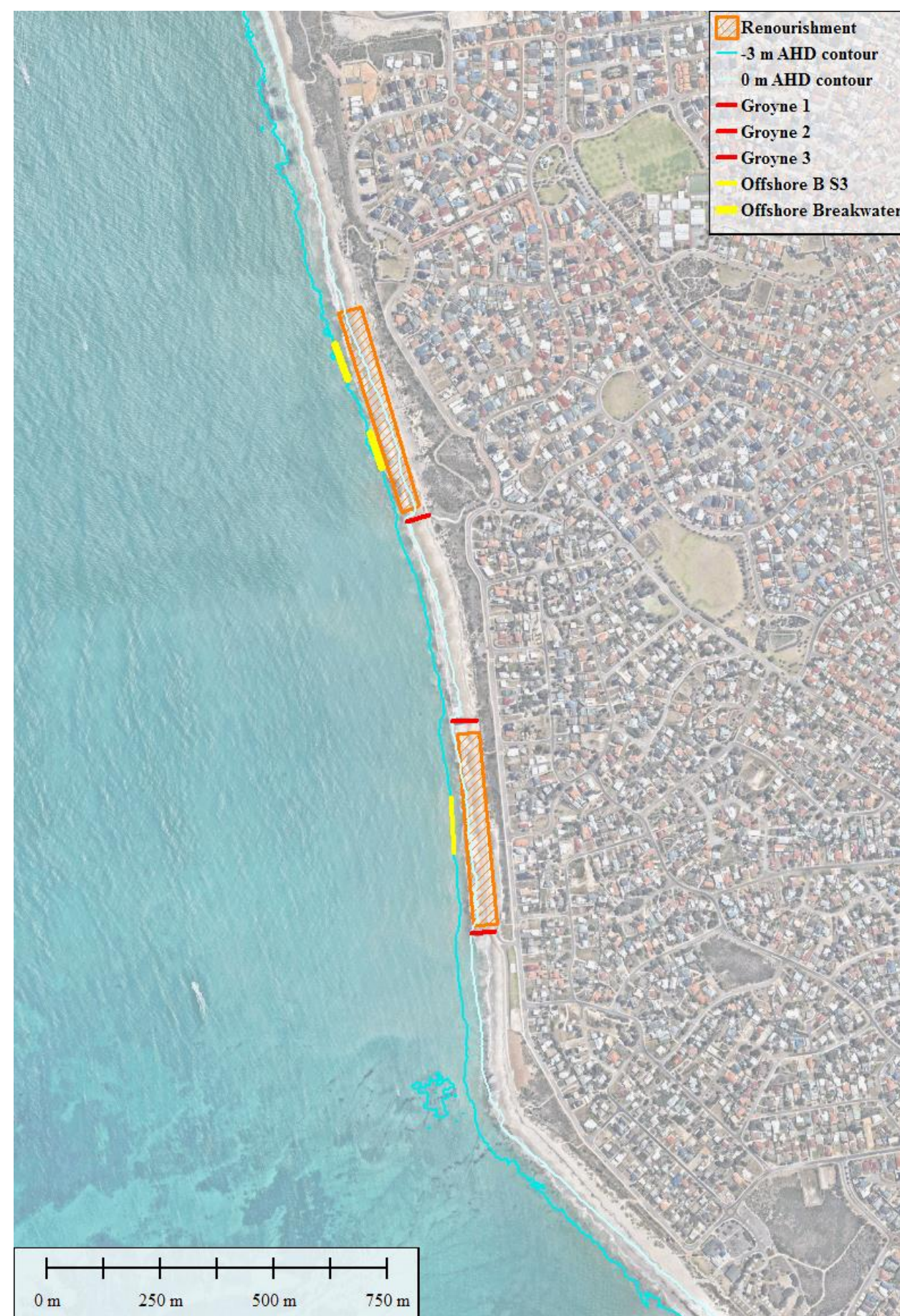
Figure 2-2 Conceptual Layouts for (a) Option 11. Groynes 1 to 3 are unchanged in length; offshore breakwaters shown in yellow. (b) Option 12. Groyne 1 unchanged in length, Groynes 2 and 3 lengthened. Groyne 4 new structure.
