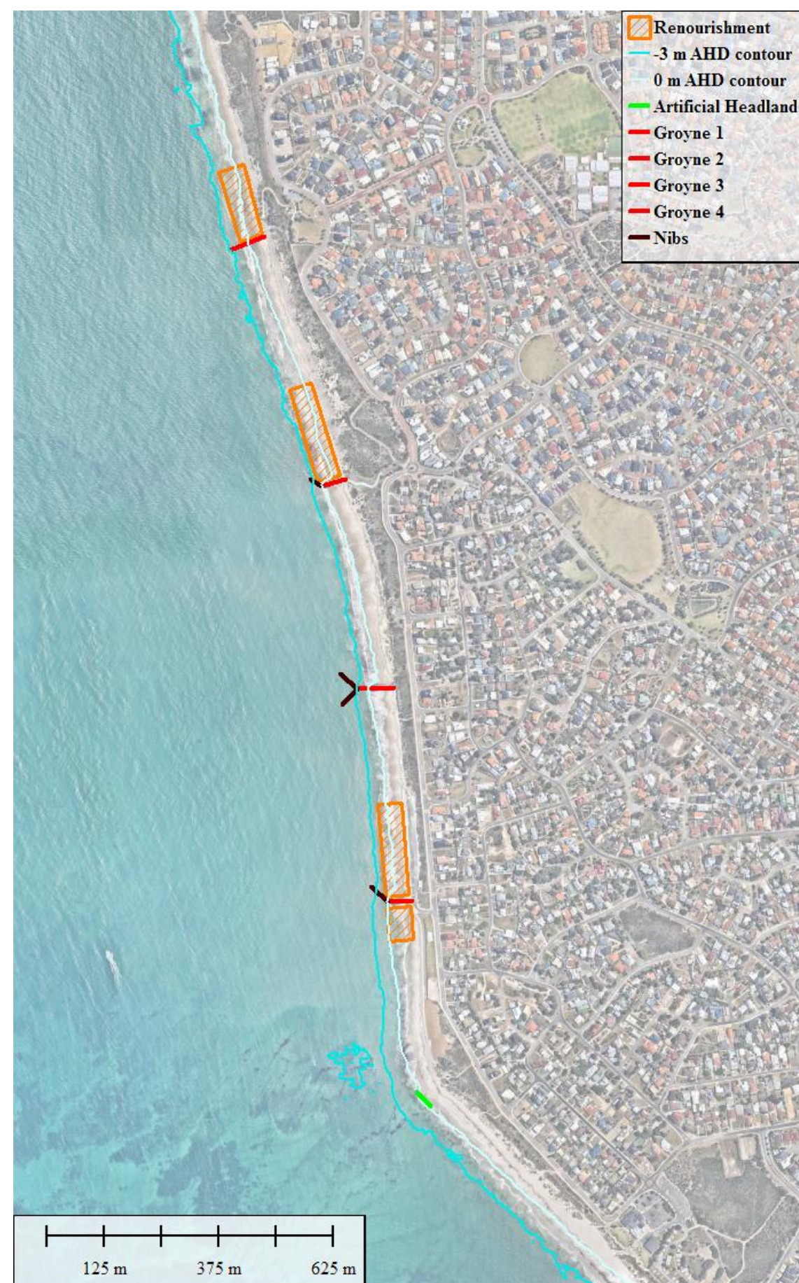
Figure 3-3 Conceptual Layouts for (a) MCA4 and (b). MCA5. Structures shown in green are existing structures; red are new / adapted structures; dark brown are breakwater nibs
