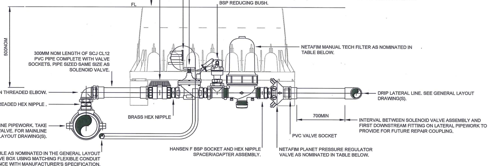
GREY MD PVC CONTROL CONDUIT WITH CABLE AS NOMINATED IN THE GENERAL LAYOUT DRAWINGS. EXTEND CONDUIT INTO VALVE BOX USING MATCHING FLEXIBLE CONDUIT WITH GLUED COUPLINGS IN ACCORDANCE WITH MANUFACTURER'S SPECIFICATION.
