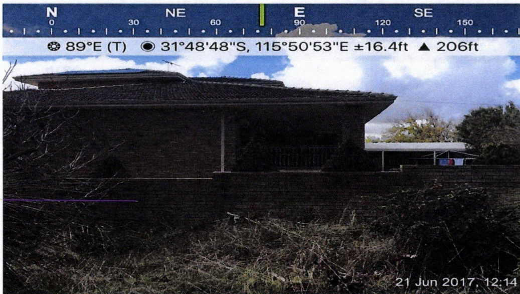
Photo Point 6: Non-vegetated and low threat areas excluded from classification under Clauses 2.2.3.2 (e) and (f) of AS 3959
