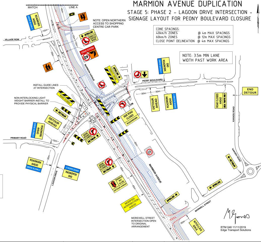
**NOTE**: CONTACT RNOC (138 111) PRIOR TO INSTALLATION OF TRAFFIC MANAGEMENT ARRANGEMENT. TRAFFIC SIGNALS TO BE SWITCHED OFF DUE TO RELOCATION OF TRAFFIC SIGNALS.
