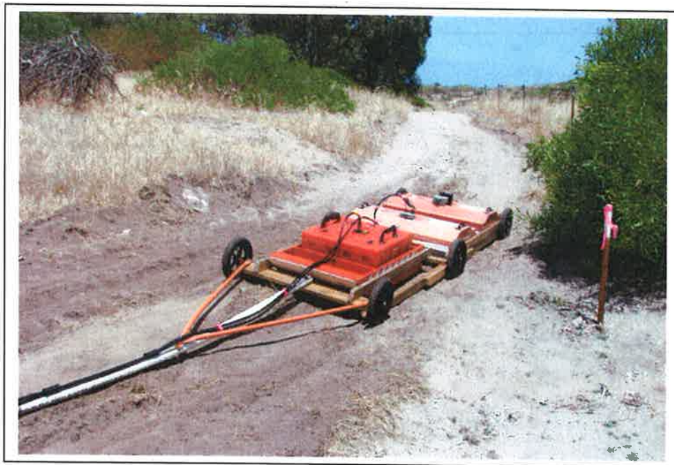
Figure 6. (Facing southwest): GPR survey trolley containing 200 MHz antenna (front) and a 100 MHz antennae bistatic pair (rear). The trolley is positioned at peg 1/1 at the start of GPR Survey Line 01, during the preliminary antenna-testing phase of the GPR survey.
