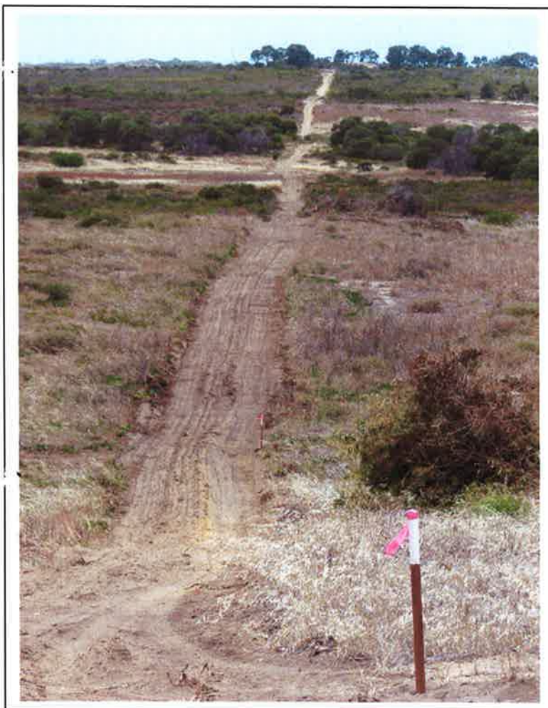
Figure 4. (Facing South) GPR Survey Line 02, starting at peg 2/20 (shown in foreground). The survey lines were prepared by lightly grading the tracks. Survey pegs were placed at nominal 100 m intervals, and at changes in direction, hill crests, or troughs.
