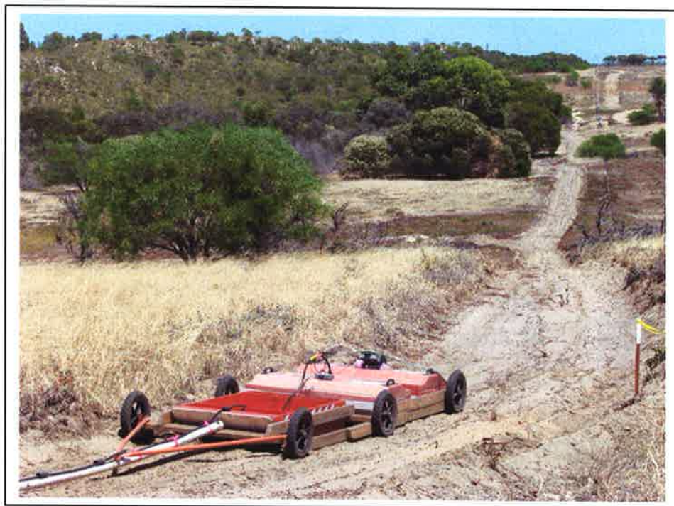
Figure 8. GPR survey trolley with bistatic pair of 100 MHz antennae as used for the production survey. The trolley is positioned near Peg 99 on GPR Survey Line 06.
