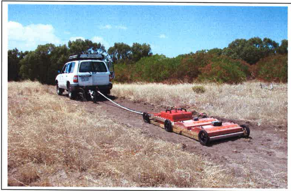
Figure 7. Antenna array with 200 MHz and 100 MHz antennae used for recording the trial GPR Survey lines. The trolley was pulled by a 4WD along the pre-graded path. Distance was measured via a survey wheel (fitted with an optical encoder) attached to the rear of the 4WD. Position marks were inserted onto the radar data as the antennae passed adjacent to the survey pegs.
