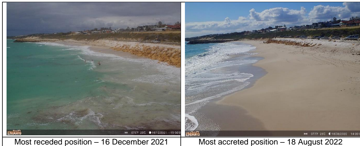
Figure 6-4 Most receded and most accreted shoreline position to the north of Quinns Groyne 1 during the study period.
