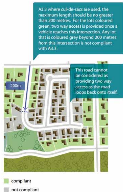
Figure 21: Example of compliant and non-compliant two-way
