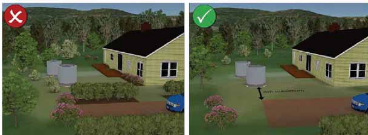
Example of good and bad landscaping around a water tank
