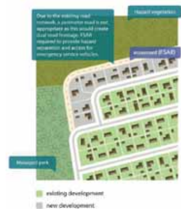
Example of Fire Service Access Way
