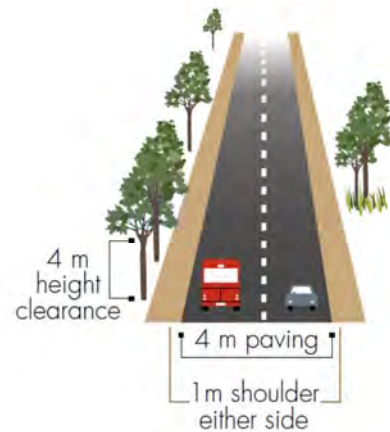
Figure 19: Minimum design requirements for a public road
