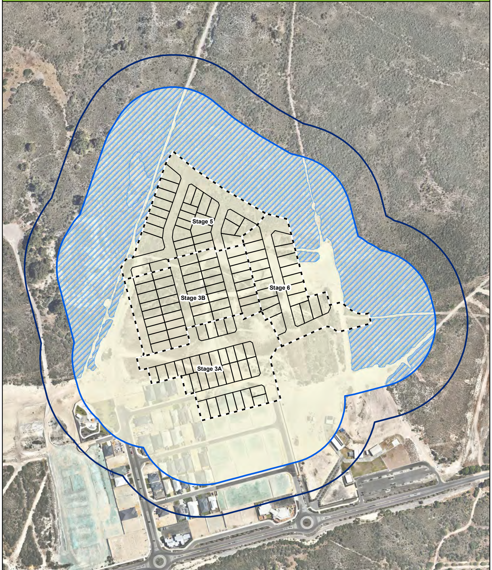
Figure 5: Bushfire Attack Level (BAL) Contour – Post-establishment of Asset Protection Zone
