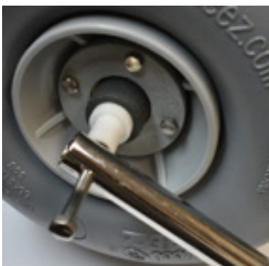
Center wheel between castor forks and install bolt
