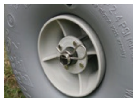
Reinstall Hitch Pin to retain wheels.
