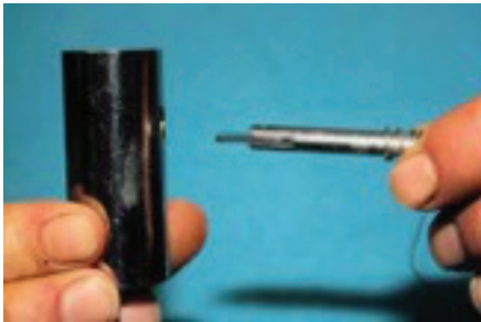
Hold latch pin in horizontal (level) position and insert into intended hole.
