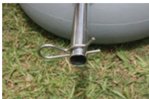
Remove Hitch Pin from axle.
