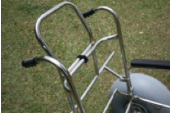
Anti-tip/ parking brake in stowed position.
