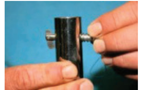
Rotate latch tab (as shown) and release.
