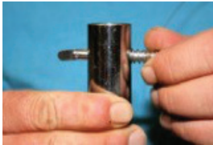
Fully compress spring and rotate pin as shown.
