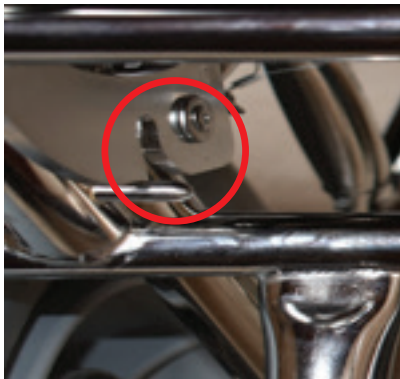
Locking bar and pin disengaged.
