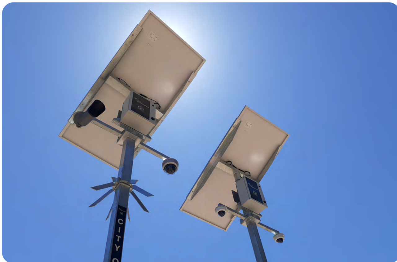
Following the problem spots. Mobile CCTV cameras are moved to areas with known antisocial behaviour every 3 months. ▲
